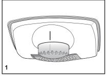
Operating temperatures are controlled by the thermostat (see diagram) located on the ceiling of fridge compartment. Settings may be made from 1 to 5, 5 being the coldest position.
